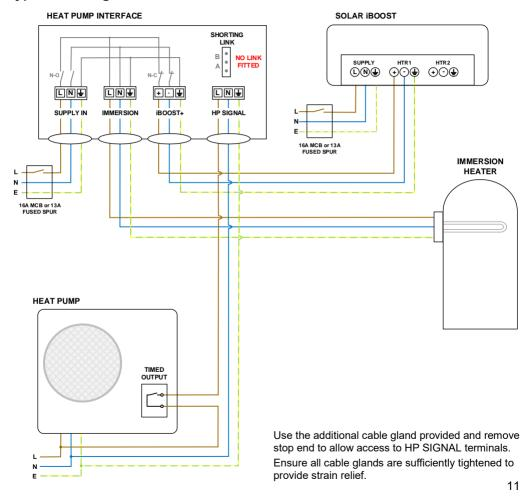
Type 5 - 230V AC 3kW supply via external relay/contactor
