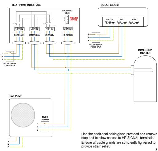
Type 2 - 230V AC 3kW output from Heat Pump
