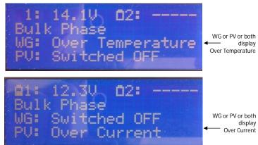
When the condition subsides the normal display is automatically resumed except in the case of PV over current. See below.
