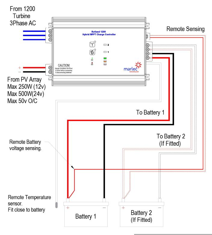
Warning! Do not exceed maximum voltage & peak power rating stated or damage will occur.
