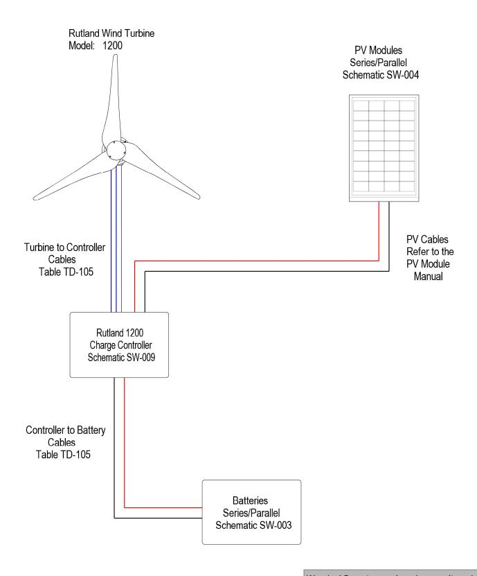
Warning! Do not exceed maximum voltage & peak power rating stated or damage will occur.
