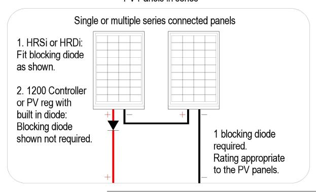
Warning! This must be read in conjunction with PV panel and regulator instructions. Do not exceed maximum voltage & peak power ratings stated or damage will occur.
