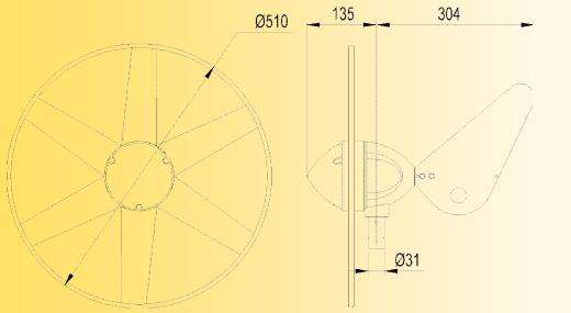
Net Weight: 3.5Kg Gross Weight: 6Kg Packing Specifications: 550x550x260mm Part No: CA-05/05 (12V)
