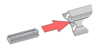
2. Slide the second BP 030 T onto the connecting kit.
