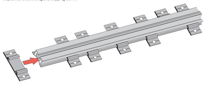
Slide the trapezoidal brackets to the correct position on the raised sections of the corrugated sheet. Adhere to the maximum spacing of 600 mm.
