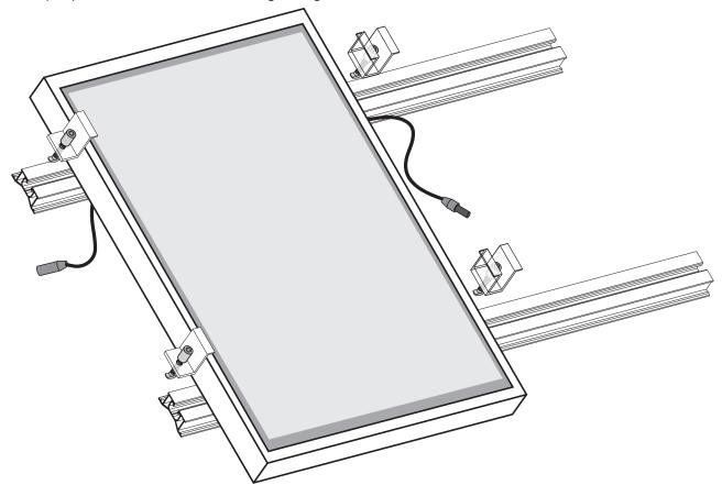
Position the end retaining clamp flush with the module frame. Lock the OneTurn in place by turning it 90° clockwise.
