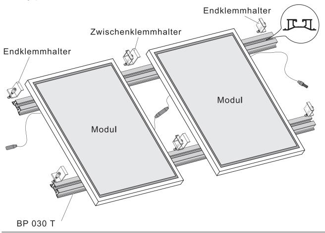
Install the modules as soon as you have installed all the required mounting rails and checked that the trapezoidal brackets are securely positioned.
