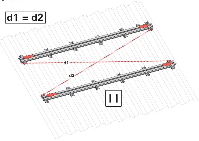
After aligning the mounting rails, screw in all the trapezoidal brackets tightly. Make sure that the mounting rails do not slip.
