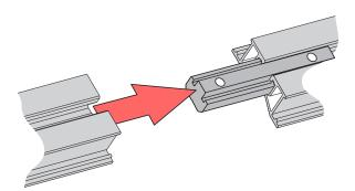
4. Tighten the punching screws of the connecting kit.
