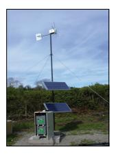
In 2007, Bristol Airport needed to supplement their airport noise monitoring system with additional monitoring locations. Suitable locations were identified but these were far away from power and communication alternatives. Estimates of over £16000 for power alone led the airport to look at an alternative approach. Additionally, it was felt that powering the equipment from renewable energy aligned very well with the environmental programmes of the airport.
