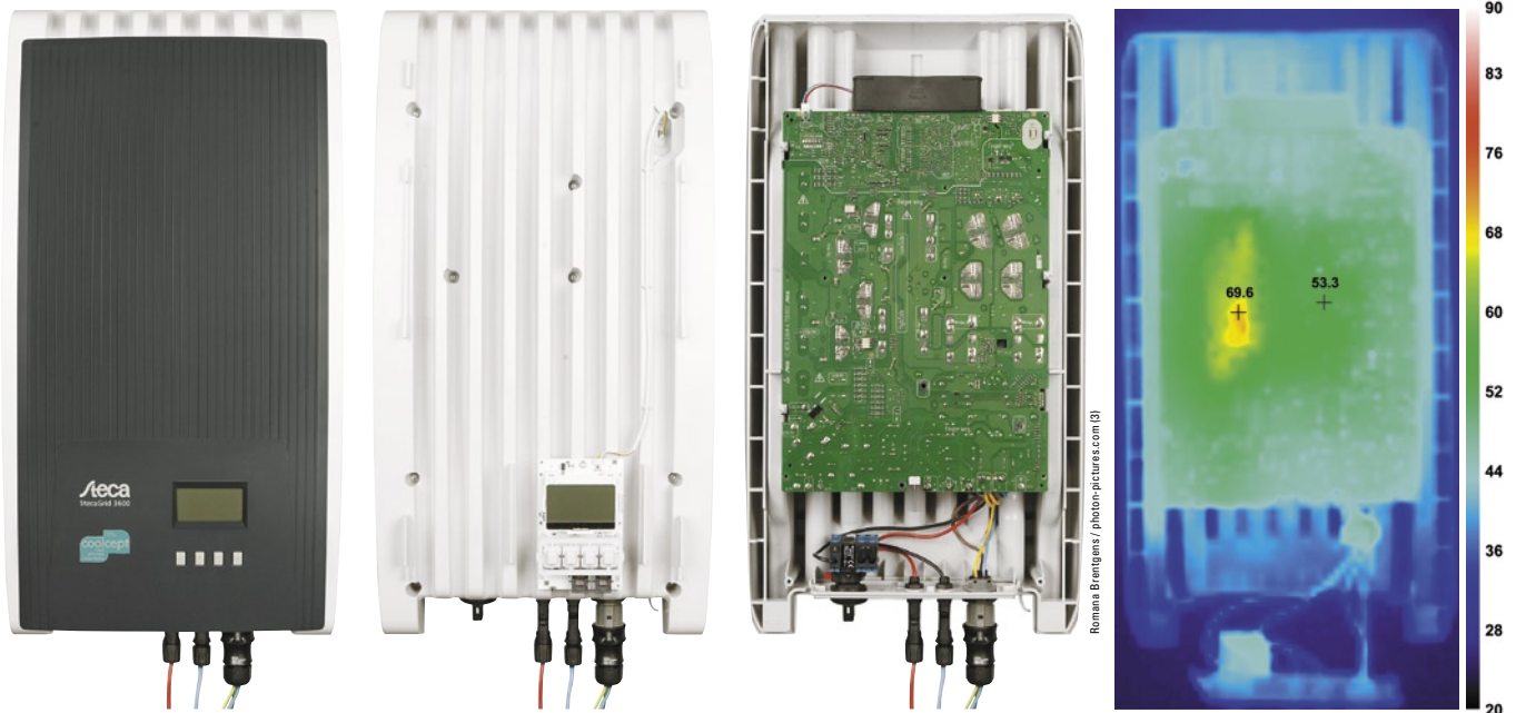
▲ Simple and cost-efficient: The Stecagrid 3600 gets by without a heavy and expensive cooling element. Its plastic housing is also cheap to produce. The thermographic imaging reveals that this concept works. While temperatures of just under 70 °C are generated close to the two buck converters during operation, it is not harmful in regard to the service life of the components.
